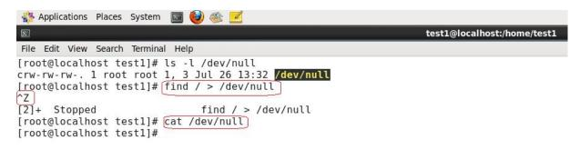
Certain commands like **find** will produce voluminous amounts of output which can overwhelm the console. To avoid this, we can redirect the large output to a special file (a device node) called /**dev/null**. This file is also called the **bit bucket** or **black hole**.
